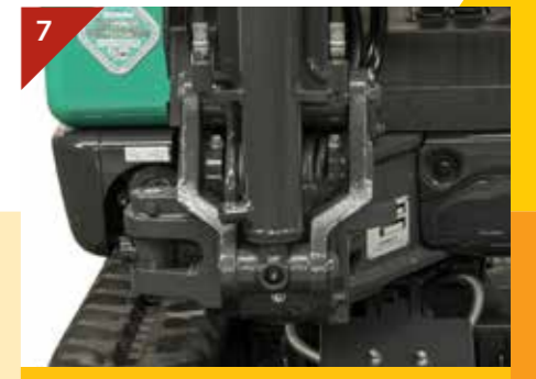
Offset boom - for increased visibility and boom rotation
