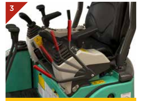
Gate lock system - Designed to lock all functions
