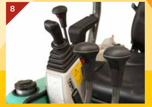
Two speed selection and track extension selection on joysticks
