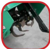
Tines operate both clockwise and counter clockwise
