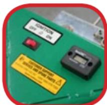
Tachometer shows engine RPM & service intervals
