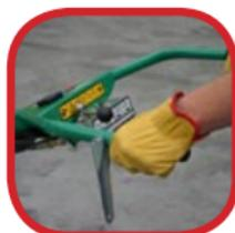
Tine, wheel drive & clutch operator controls
