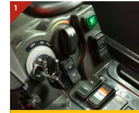
Centralised switches - includes key start, throttle dial, auto idle & eco mode
