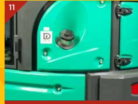
Fuel refill located in a convenient position
