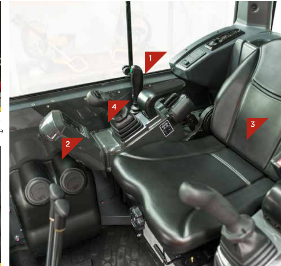
Easily visible monitor - includes travel speed, auto idle, eco mode, hour meter & engine management
