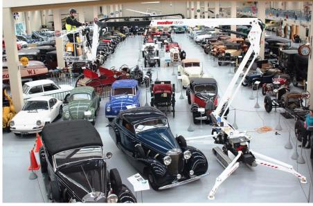
The 1575 is an extremely compact Spider Lift for the most difficult applications. The track system expands out to 1060 mm for extra stability and stands taller for extra ground clearance.
